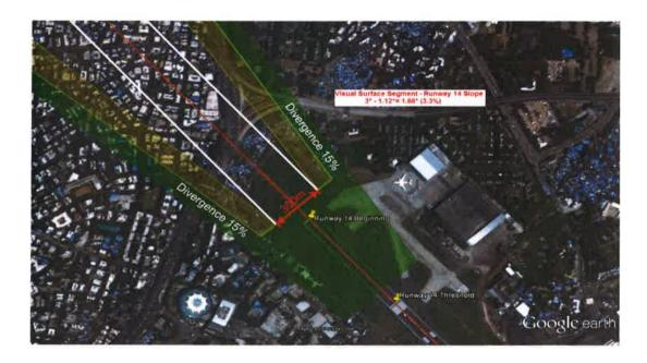
Hence, the required obstacle protection slope of 3.3%(1:33.33) for VSS area is not protected which is a safety hazard as the obstacle are not protected or limited in respect to threshold (Displaced).
