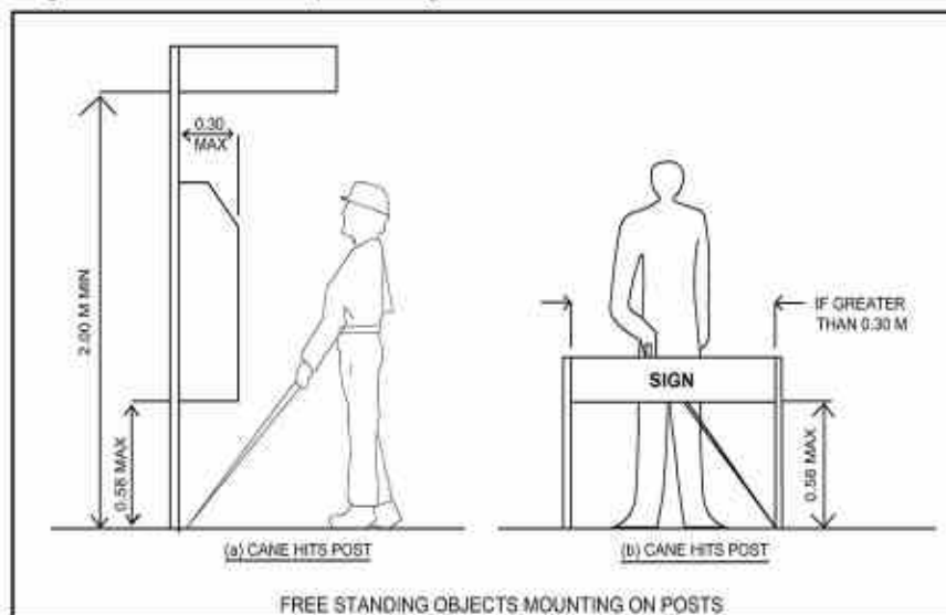
Figure No. 41. Limits for protruding obstructions.
