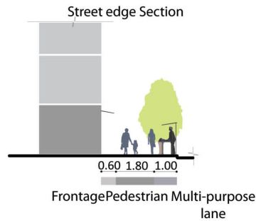
Figure No. 11. Street edge design section
